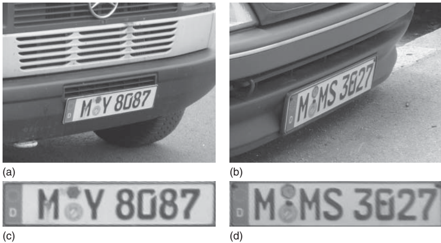
Figure 9.20 (a,b) Images of license plates. (c,d) Result of a projective transformation that rectifies the perspective distortion of the license plates.
