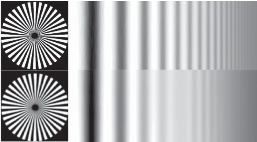
Figure 1.4 Spurious resolution. The modulation transfer function (Figure 1.3) shows oscillations beyond the cutoff spatial frequency, which show up in defocused gratings as contrast reversals. On the left, a circular grating shows the contrast reversals at the higher spatial frequencies in the center (top: in focus, below: defocused). On the right, the grating shown in Figure 1.3 was defocused. Note the lack of contrast at the first transition to zero contrast, and the repeated subsequent contrast reversals. Note also that defocusing has little effect on low spatial frequencies.
