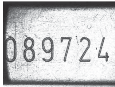
Figure 3.76 Highly specular surface with engraved characters. Only at the perfect reflecting surface parts the image is bright. Disturbing structures destroy the telecentric characteristics of light. So the characters appear dark.
