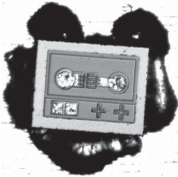
Figure 3.72 The diffuse incident lighting levels differences of brightness from tooling marks on the test object surface: chip stuck on to an aluminum sheet.
