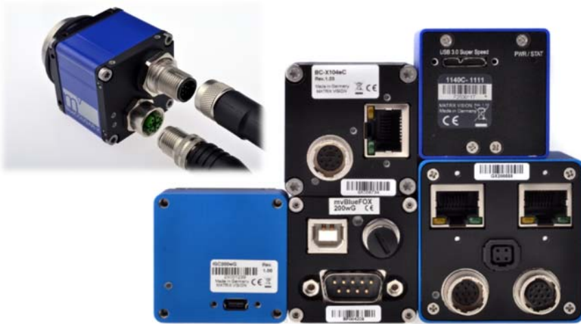
Figure 6.72 Upper left: Industrial M12 option with x-coded GigE and IO; lower left: mini USB2; lower middle: USB2 Type B; upper middle: RJ45 and HiRose; upper right: micro USB3; lower right: dual RJ45 plus dual HiRose (motorized lens control) and video lens control.
