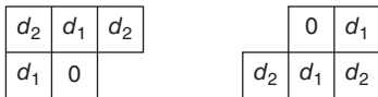
Figure 9.57 Masks used in the two sequential scans to compute the distance transform. The left mask is used in the left-to-right, top-to-bottom scan. The right mask is used in the scan in the opposite direction.
