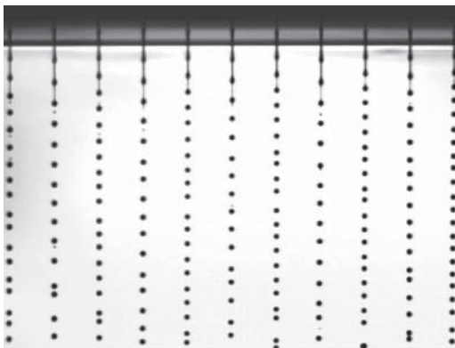
Figure 3.104 Edge triggering with very low delay times allow us to achieve flashes from 0.5 to 100\ \mu\text{s} that are able to image blur free object speeds up to 30\ \text{m s}^{-1} . The image shows ink drops that are injected under high pressure.
