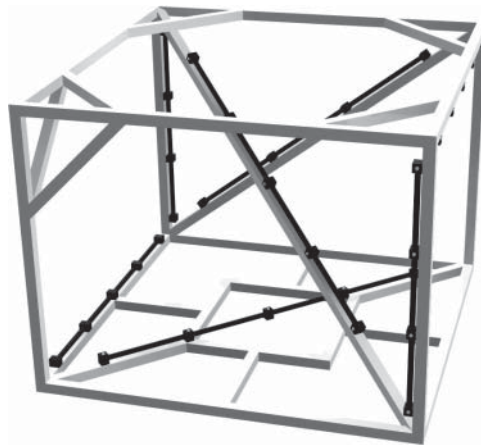
Figure 5.14 Spatial test object for VDI 2634 test.
