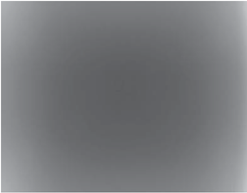
Figure 3.51 Brightness profile of a lighting to compensate natural vignetting of an imaging objective.
