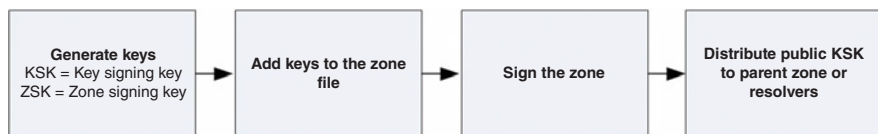
Figure 9.2. Basic DNSSEC Implementation Steps
