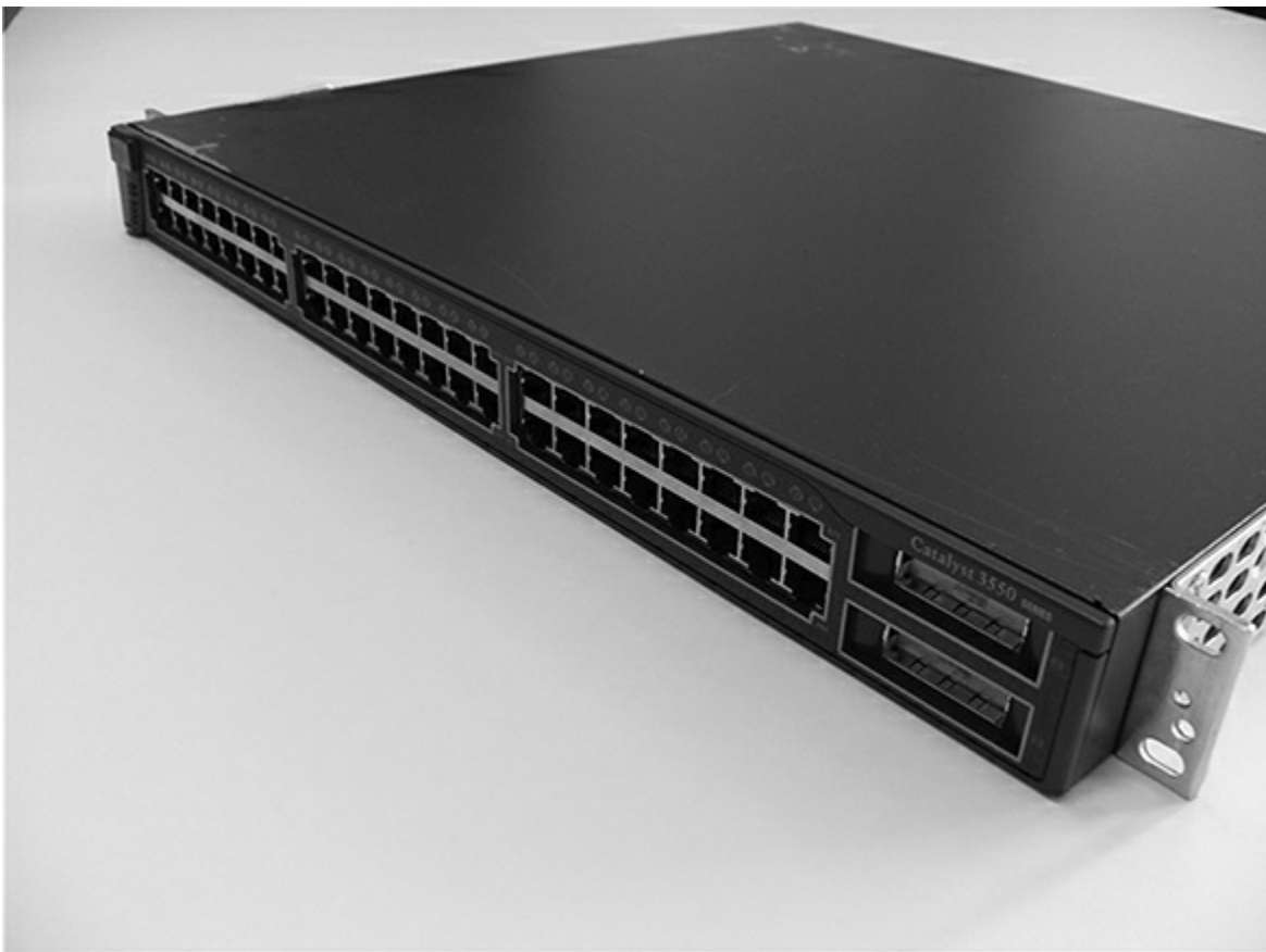
Figure 3.14 An Ethernet layer 3 switch.
