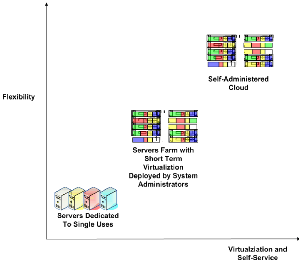
Figure 5.2: The greater the virtualization and support for self-administration, the greater the flexibility in adapting computing resources to changing service needs.
