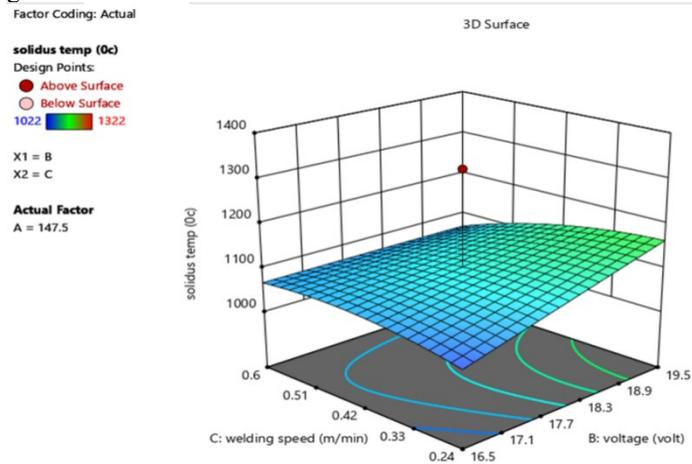
Figure 4: Solidus temperature, voltage and welding speed
