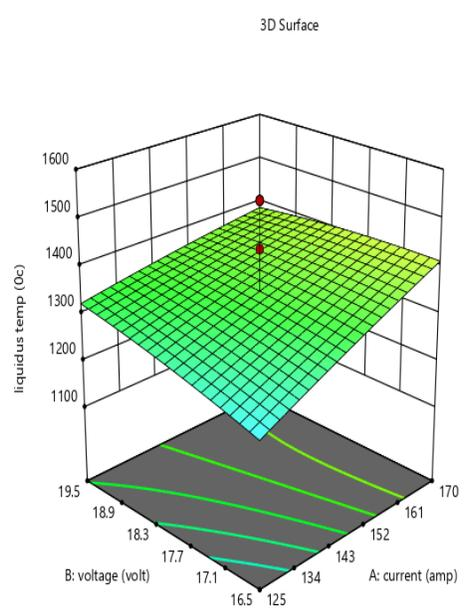
Fig. 1: Surface plot for Liquidus temperature, current and voltage
