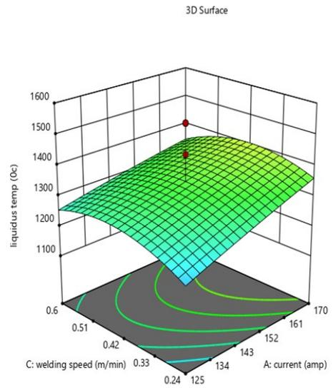
Fig 2: Liquidus temperature current and welding speed
