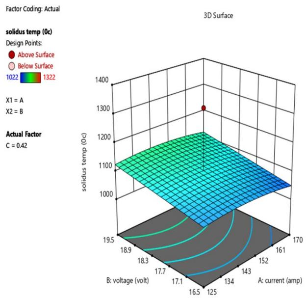
Figure 5: Solidus temperature, voltage and Current
