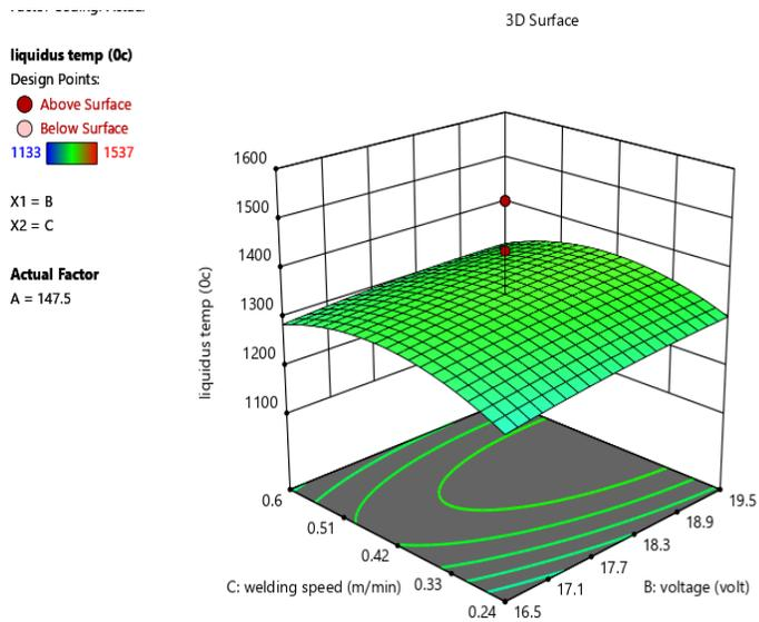
Fig. 3: Liquidus temperature, voltage and welding speed
