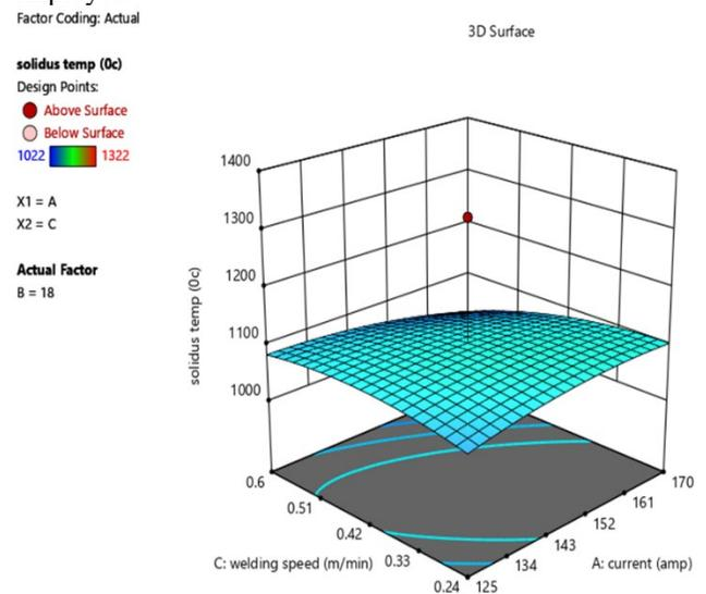
Figure 6: Solidus temperature, welding speed and Current
