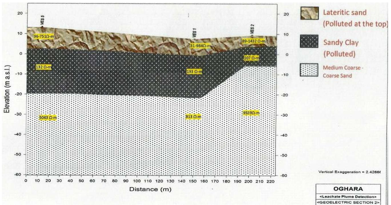
Fig. 6: The Geoelectric Section Connecting VES 1, VES 3, VES 4 and VES 6
