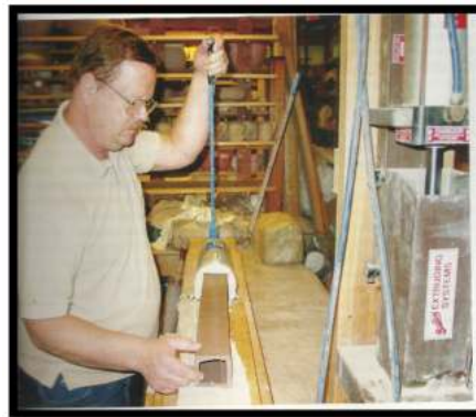
Figure 1: A Hand Extruder Mounted on a Hinged Board Extruding A Hollowed Squared form Designed by Tim Frederick Source: Speight and Toki (2004:537)
