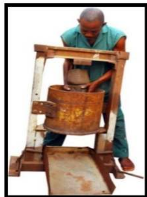
Figure 19: Loading of Clay into the Feeder Trough
