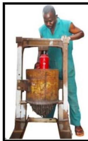
Figure 22: The Equipment in Operation Extruding 220 Slab-Strips at a Time
