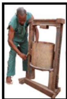
Figure 14: Fixing and Screwing of Feeder Trough with Seventeen Sized Bolts, Washer and Nuts on the Frame
