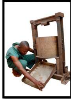
Figure 15: Fixing of the Collection Trough
