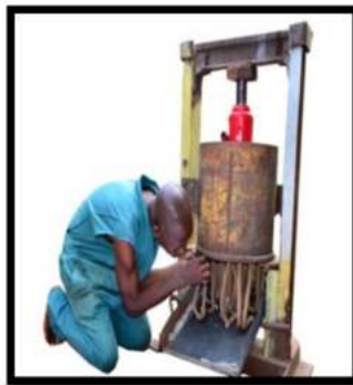
Figure 21: Cutting out Extruded Slab-Strips
