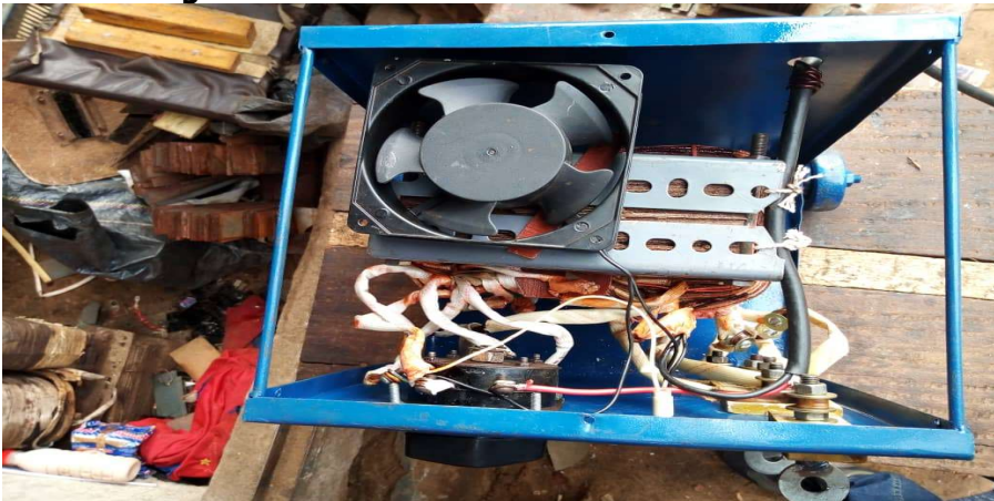
Plate 2: Pictorial View of Fixed Air Blast Cooling System
