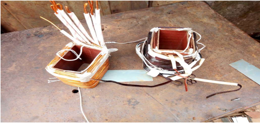
Plate 1: Pictorial View of Assembled Windings 3.2.3 Cooling
