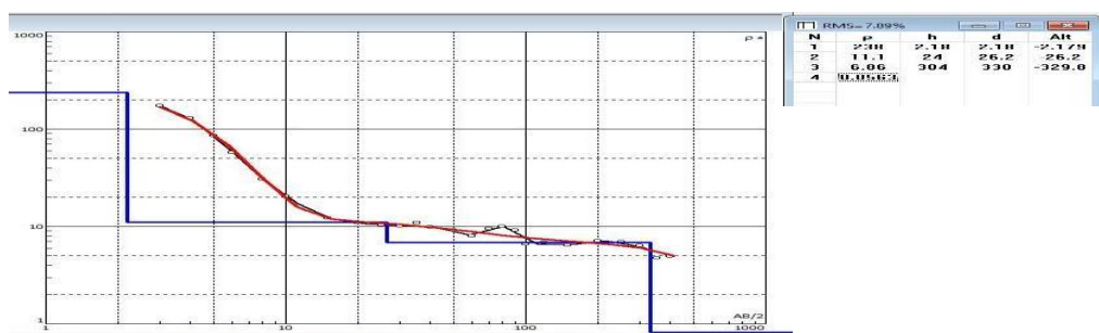
Figure 4: Resistivity sounding curve for Ndi Agbo Community School,
